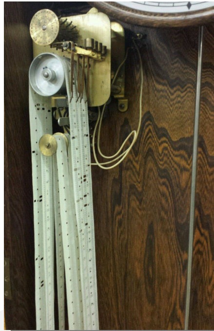
Paper Tape Programmable Control
