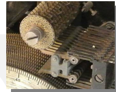
Pins on Discs to set on/off times & days
